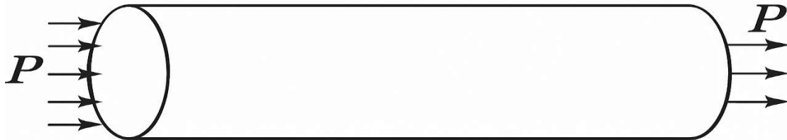
Figure 1. Cylindrical shell that can withstand extreme compressive loads.
