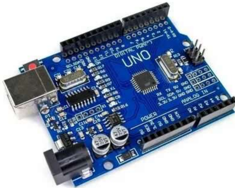
Figure 1. Appearance of the Arduino board Uno
