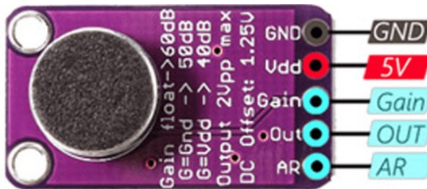
Figure 6. Pinout sound sensor MAX9814
